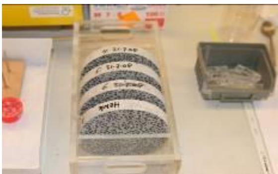
Concrete cylinder: cut in slabs
