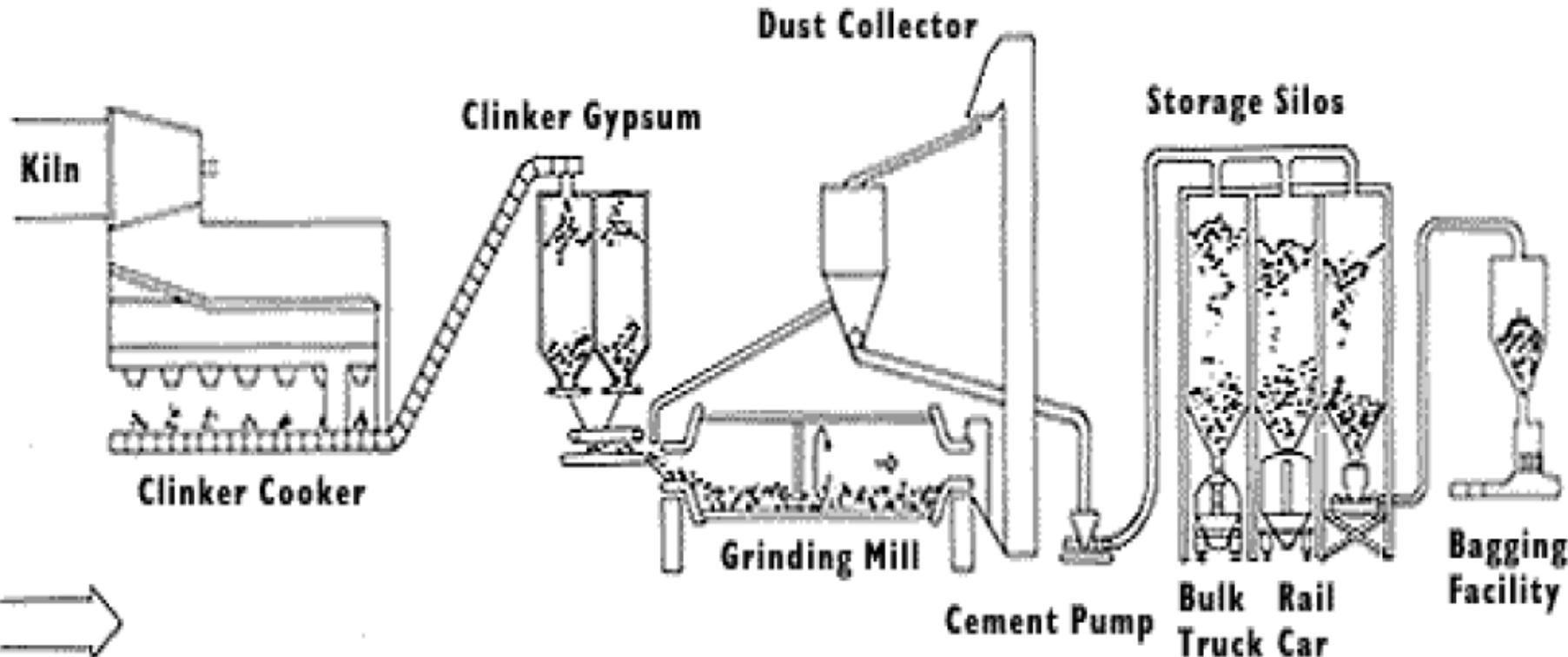
Once cooled, the clinker is ground with a small amount of gypsum.
